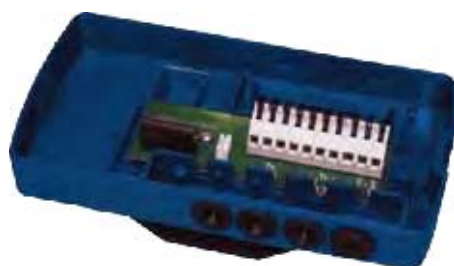
Sockets for temperature sensors and the volume meter
