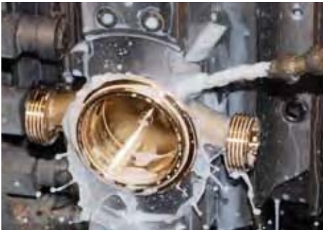
Machining on transfer machine
