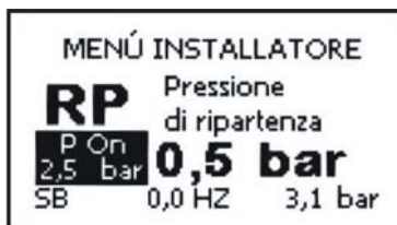
Figure 13: Setting the restart pressure
