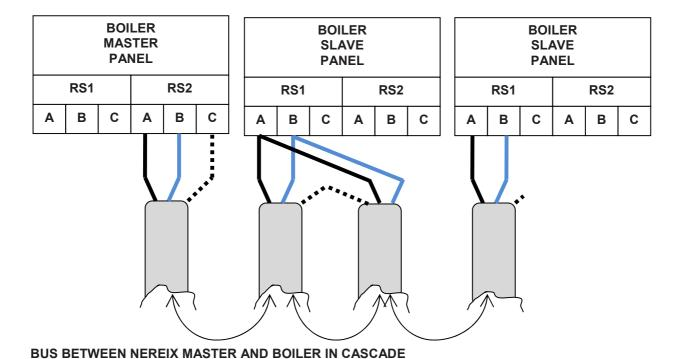
The RS1 C contact (corresponding to terminal 34) is only for support of the cable shield; it is not necessary to connect it to the last slave.
