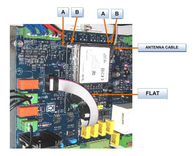
The standard antenna can be mounted inside the panel (with its double-sided adhesive) or put on the outside in a manner consistent with the length of the cable provided.
