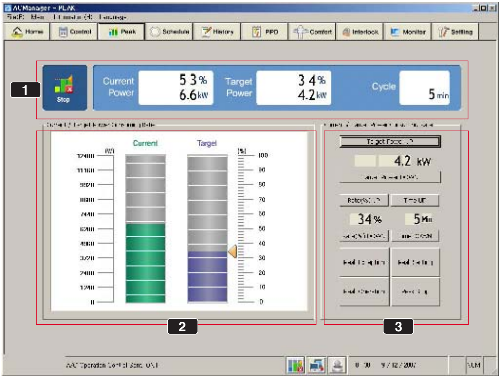
(1) Current operation status & power control setting
