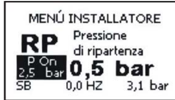
Figure 17: Setting the restart pressure
