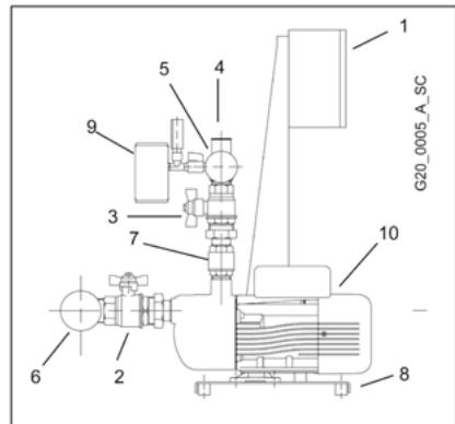
The check valve may be located on the delivery or suction side, depending on the type of set; the electric pump may be vertical or horizontal type.
