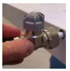
**Notice!** The connection pipes are internally soft-welded why it's not allowed to solder the beam to the pipes.
