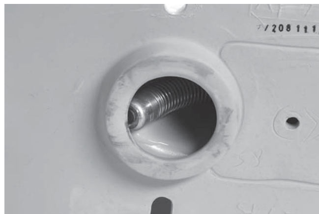
Figure 20 – Camera Head Blocked in Turn
