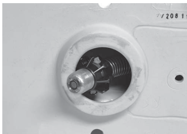
Figure 21 – Camera Head with Ball Guide in Turn
