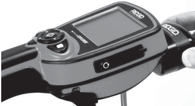
Figure 10 – Connecting the microEXPLORER Camera Monitor
