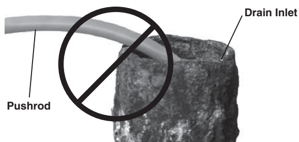
Figure 18 – Avoid Pulling At Sharp Angles
