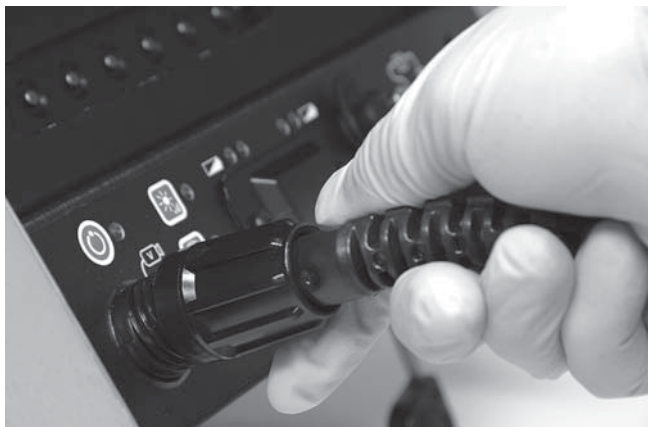
Figure 13 – Connecting To A SeeSnake CCU
