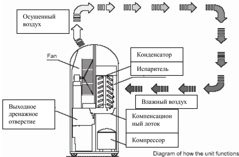
Diagram of how the unit functions
