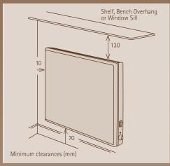
The recommended height off the floor is a minimum of 70mm. The sides of the panel heater can be installed within 10mm of a corner or furniture located against a wall. Directly under windows is an ideal location.
