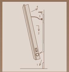
The bracket design allows the panel heater to be unclipped and tilted forward for cleaning and access to the power point.
