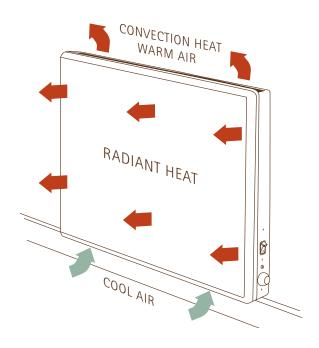
Just like the sun, radiant heat is multi-directional, and works on the principle of warming surfaces and objects within a room. Radiant heat is universally regarded as a very efficient, healthy and comfortable method of heating.
