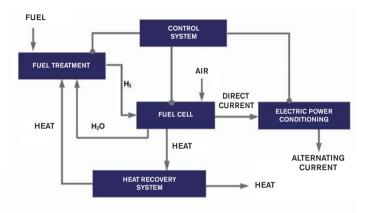
Scheme of a unit with fuel cells
