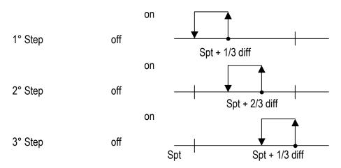
N.B: the number of steps controlling the cooling tower is selectable by keypad under "User" password.
