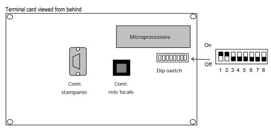
The address of the terminals is set up through the dipswitch bench found on the back . The address is selectable in the 1-16 range by utilising the 1-5 dipswitch. The address value is obtained via the following table (see also previous paragraph):
