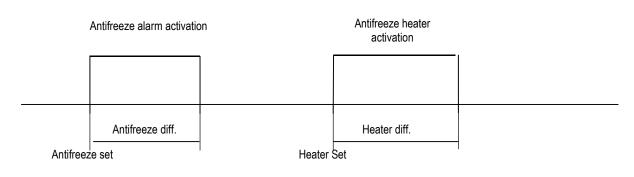
The antifreeze regulation is always energized also when the machine is OFF, both summer working and winter working.
