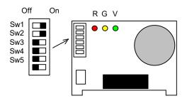
In the standard application EPSTDEMCHA modular chiller addresses for the MicroTech II units:
