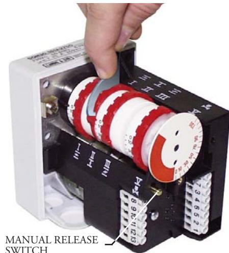
Remove cover to gain access to the adjusting cams. The cams are to be adjusted through the suitable key provided for. Description:
