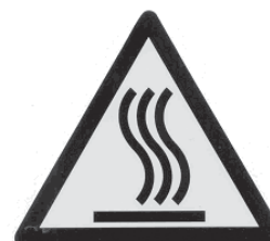
Warning - high-temperature zones Adjacent to hot pipes or components
