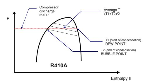
The difference between the Dew Point and Bubble Point is known as "GLIDE" and this is a characteristic property of refrigerant mixtures. If pure fluids are used, the phase change occurs at a constant T and thus the glide is equal to zero. If HFC R410A [ 50%-50% blend of R32 and R125] is used, the glide will be negligible  $(0.2^{\circ})$  and the fluid can be considered like a pure fluid.
