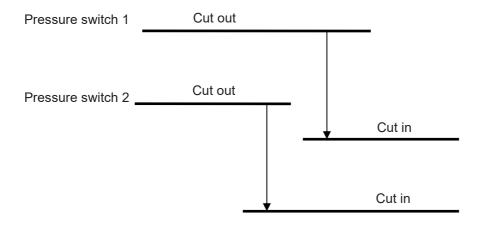
...where <u>pressure switch 1</u> is set at the "PS" (maximum admissible pressure) of the system, while <u>pressure switch 2</u> will have the setting = PS x 0.9 in accordance with the reference technical standard.
