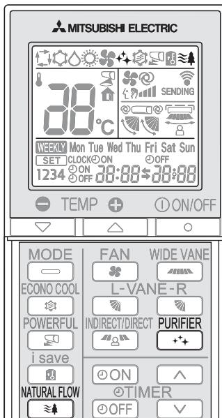
Press **NATURAL FLOW** during COOL or FAN mode [page 6](#) to start NATURAL FLOW operation.
