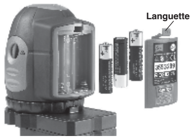
Figure 4 Installation des piles
