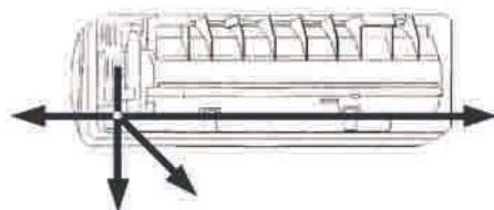
Possible outlets of hydraulic pipes
