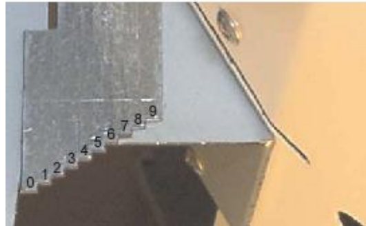
Step indicators showing the position of each regulating screw.
