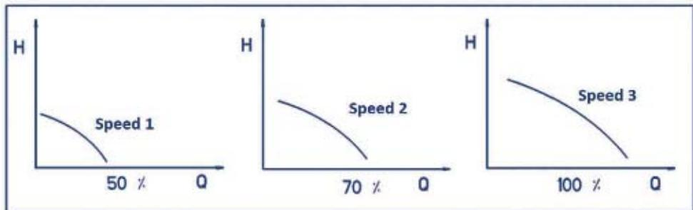
Fig 9: Characteristics of the pump at different speeds
