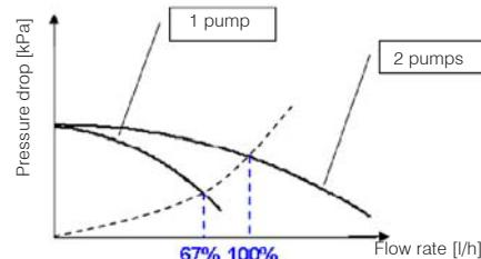
In the case of two pumps in combination, the advanced microprocessor is mandatory because it controls the on/off switching of the second pump according to the number of capacity steps required at every instant. This makes operation of the unit cost-effective for most of its life since, based on well-known analyses, chillers operate 97% of the time under part load conditions.
