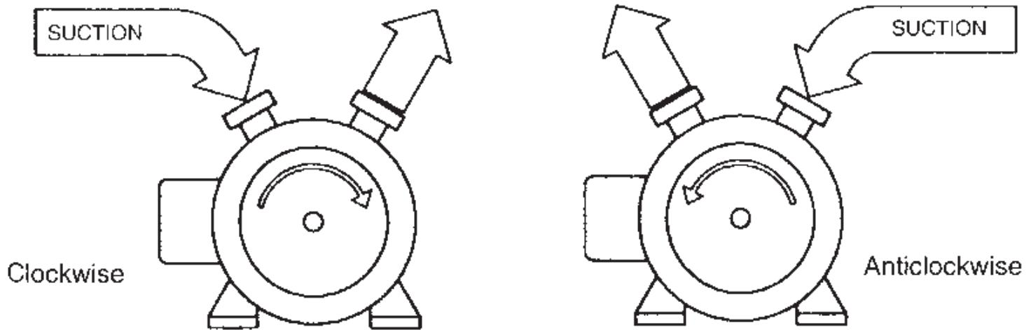
**Hose connection** - Before connecting the hoses, pour into the body of the pump some of the liquid to be transferred, in order to fill up half of the total capacity. This must be done to get the priming, that is the suction of the fluid, automatically carried out by the pump while it is working. Then, connect the hoses, that shall be either rigid or stiffened, securing them to the hose fittings using hose-clamps.
