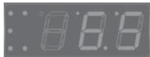
Press once to **reset** all **manually reset alarms** not currently active; all the alarm events per hour will also be reset even if the alarms are not active. Hold down the key for **2 seconds** to turn the Chiller from on to off or vice versa. When it is off, only the decimal point remains on the display.
