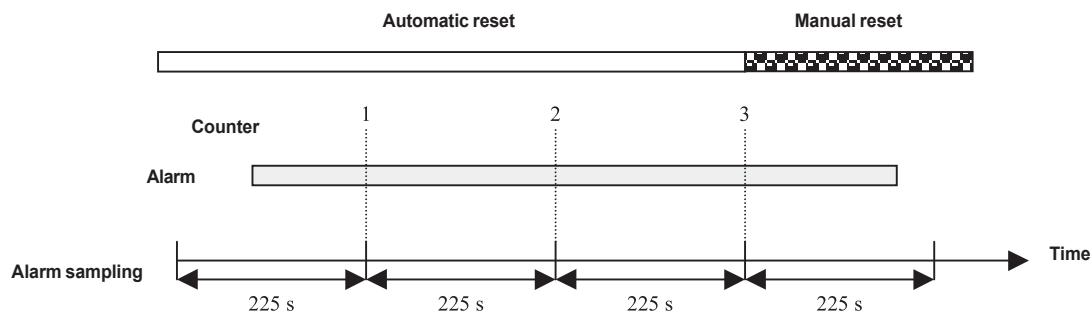
If an alarm is triggered more than once within one sampling period (226 seconds), only one alarm will be counted.
