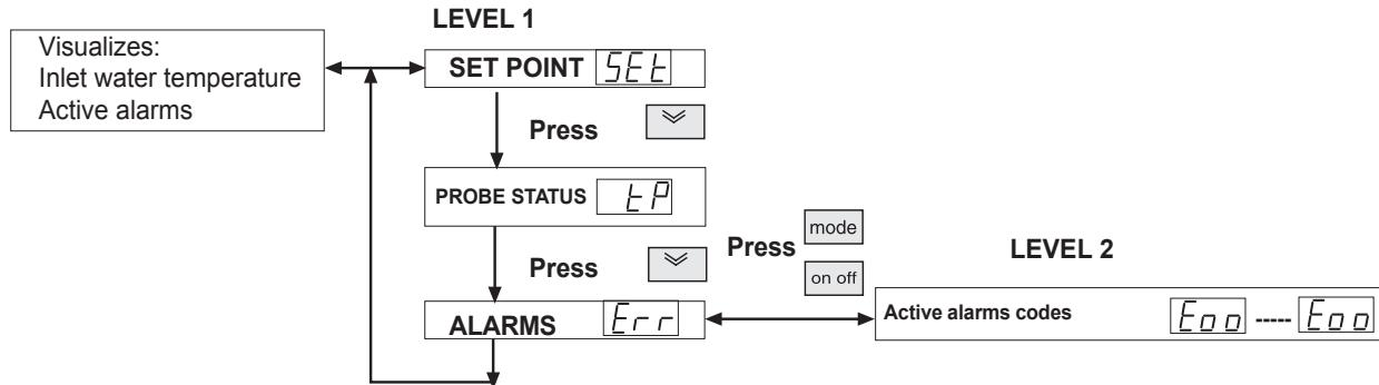
The unit self-protect through safety devices, when any of these safety devices detect an anomaly, shown in the display in order to advice the installer.
