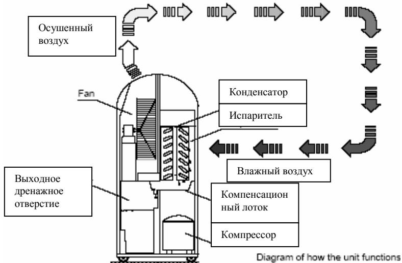
Diagram of how the unit functions
