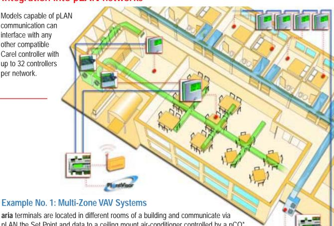
pLAN the Set Point and data to a ceiling mount air-conditioner controlled by a pCO\*. The pCO\* uses this information to manage the temperature and humidity in the building by meeting each room's demand.
