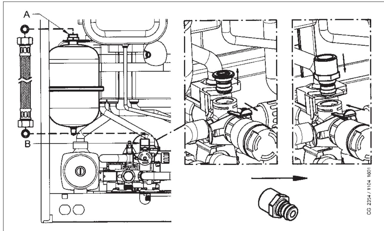
Connect the hose (supplied as an accessory in the expansion vessel kit) to the two connectors A and B as shown in figure. The DHW expansion vessel should be mounted if:
