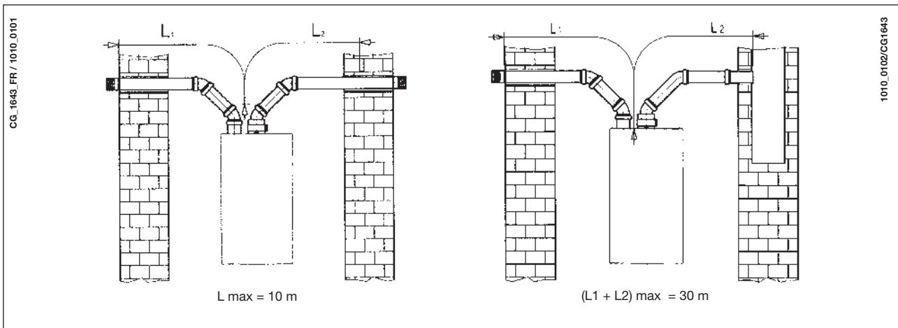
**N.B.:** For the C52 type, do not fit the flue and air duct terminals on opposite walls of the building. The inlet flue must have a maximum length of 10 metres for C52 fumes outlets.
