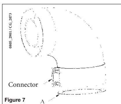
If fumes are discharged outside the building, the flue-air duct must protrude at least 18 mm from the wall to allow an aluminium weathering surround to be fitted and sealed to avoid water infiltrations.
