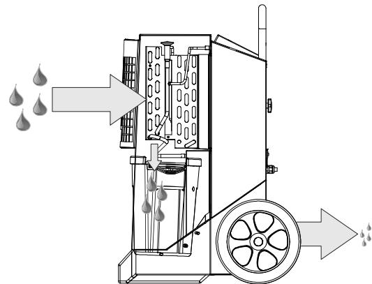
As the air is repeatedly circulated through the dehumidifier, its moisture content is repeatedly reduced, resulting in rapid, gentle drying. The dehumidifier can run constantly, or be controlled by a built-in hygrostat.
