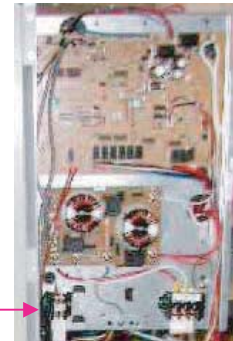
Figure 6.1 Resistance measurement between A-B of super-link signal wire (Confirm if there is entanglement between signal wire and power wire)
