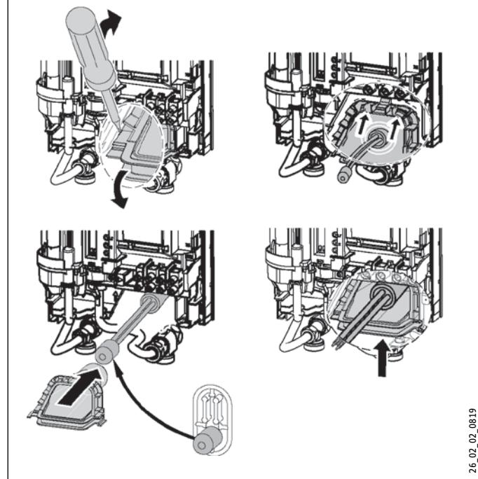
If cables with a large cross-section are used, the cable grommet can be fitted after the appliance has been installed. Take the following steps:
