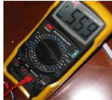
Step 2: Check the voltage between the two electrolytic capacitors, the normal value should be 510V~580V.
