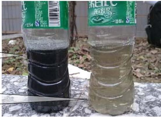
The oil is still transparent, but there is impurity in the oil, the impurity may clog the filter
