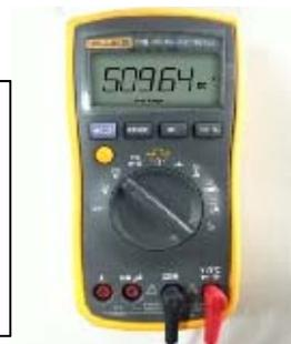
If the value is not in the range, that means the power supply for electrolytic capacitors has problem, you should check the power supply, whether the voltage is too high and whether the voltage is stable.
