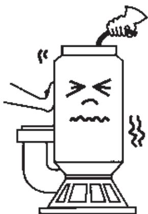
(4) Do not move pump by pulling the cable. It may lead to breakage in the cable core, decrease the insulation and cause the leakage of electricity.
