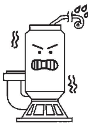
Do not extend the cable freely and submerge the electrical joint into water.
