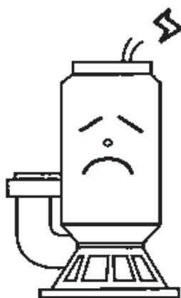
No buzzing and failure in running after switch on the power
