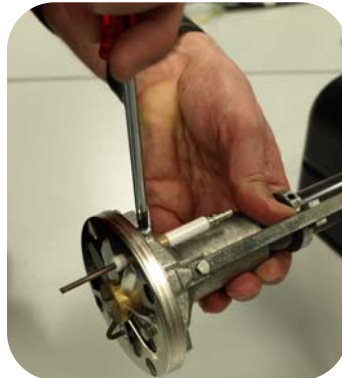
6-Unscrew the fixing screw of the ionization electrode and remove it.
