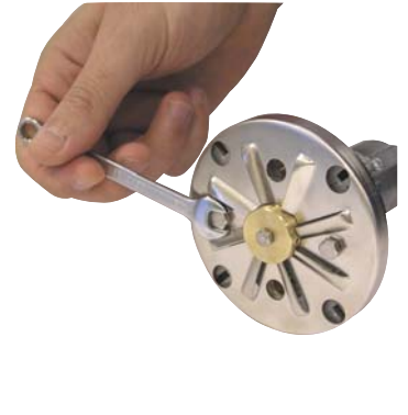
8-Unscrew the two fixing screws and remove the diffuser (spanner 8 mm).
