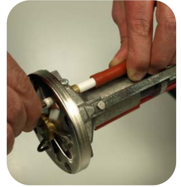
4-Remove the cables of ignition and ionization.
