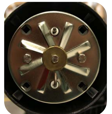
12- Reassemble the blast tube in the burner.
