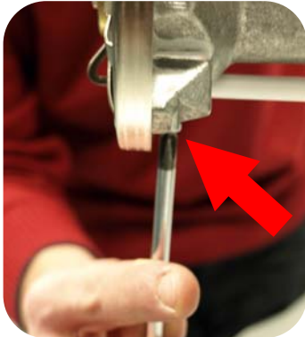
5-Unscrew the fixing screw of the ignition electrode and remove it.
