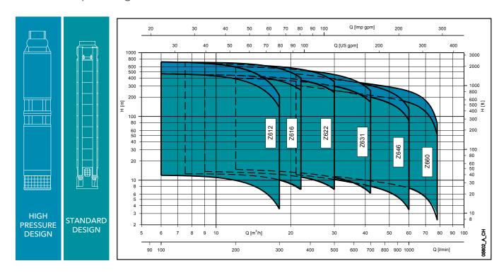
Z6 series operating characteristics at 60 hz.
