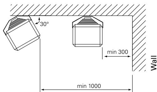
Fig. 1b: Minimum distance wall
