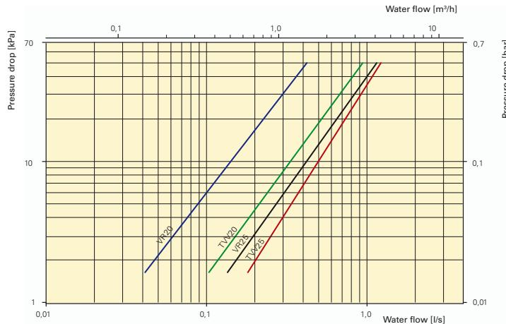
The pressure drop is calculated for an average temperature of 70°C (PVV 80/60). For other water temperatures, the pressure drop is multiplied with the factor K.
