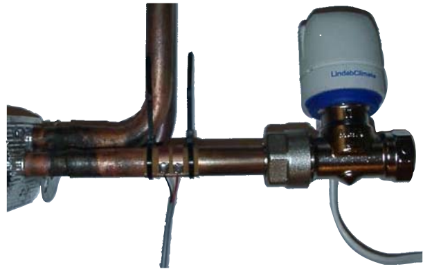
Figure 4. Sensor mounted around a horizontal, plain copper pipe and secured with two stripes
