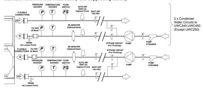
**CAUTION** Constant water flow MUST be maintained. Variable water volume is NOT recommended.
