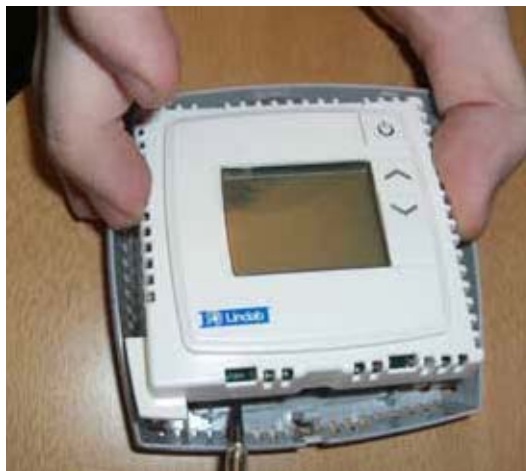
2. Remove the front including the circuit board
