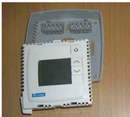
4. Remount in inverse arrangement when the plinths are connected. Notice that the front and bottom plate only can be fitted to each other in one way. See mark "UP".
