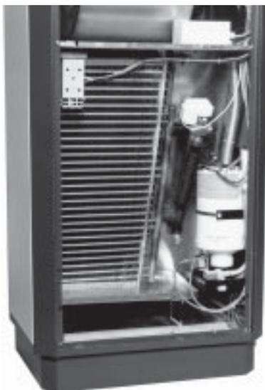
– The unit tray condensates drain must have a siphon designed in accordance with good engineering practice (the retention height must equal twice the depression value of the unit). A diam. 16 mm annulated smooth flexible hose is supplied with the unit for connecting the drain. For the siphon, a wide enough opening will be made with the flexible hose.
