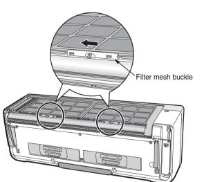
2 Slide the buckles of the filter mesh leftwards to lock the filter mesh. (Each in both sides)
