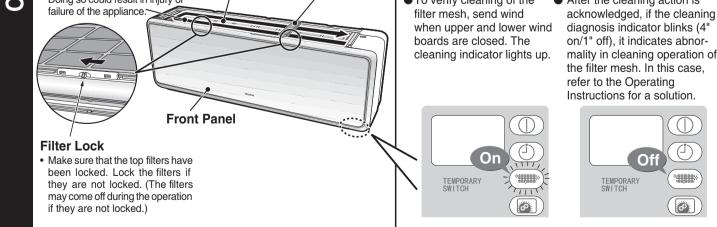
Filter cleaning operation check will take approximately 5 minutes for the cleaning unit to make one cycle of back and forth movement. Make sure that the cleaning unit is actually working by a visual inspection from the top of the indoor unit.
