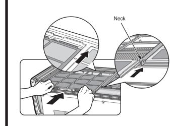
1 Keep the filter mesh facing up, and align the filter with the top face of the indoor unit, and then slide and push it in. (The shape of the left and right filters are the same.)
