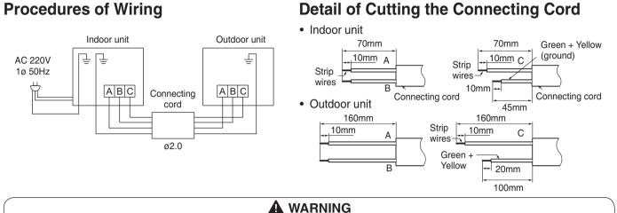
If the supply cord is damaged, it must be replaced by a special cord (Maker's service parts) available from the manufacturer The naked part of the wire core should be 10mm fix it to the terminal tightly. Then try to pull the individual wire to check if the contact is tight. Improper insertion may burn the terminal.
