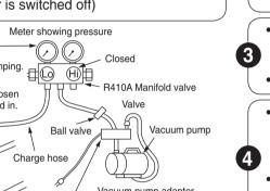
core and connect the charge cap for the service valve at large Connect the vacuum pump adapter to the vacuum pump and connect the charge hose Cap of valve core to the adapter. Loosen the spindle of the service valve with small diameter by 1/4 turn and tighten the spindle immediately after 5 to 6 seconds.
