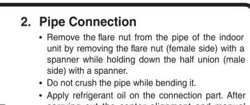
carrying out the center alignment and manual tightening of the flare nut, tighten the flare nut securely with a torque wrench (spanner).
