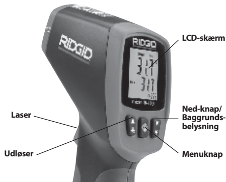
Figur 8 – micro IR-100-display/Knapper
