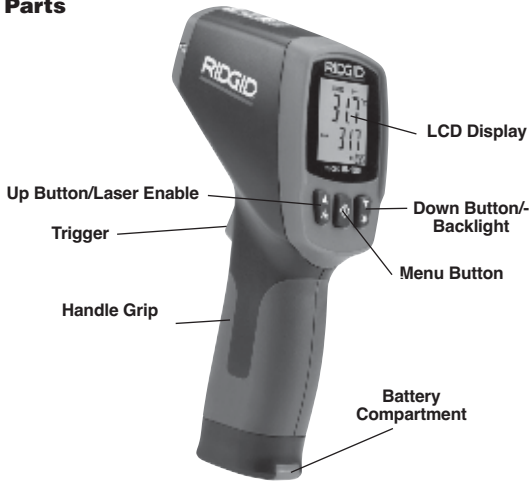
Figure 2 – micro IR-100 Parts
